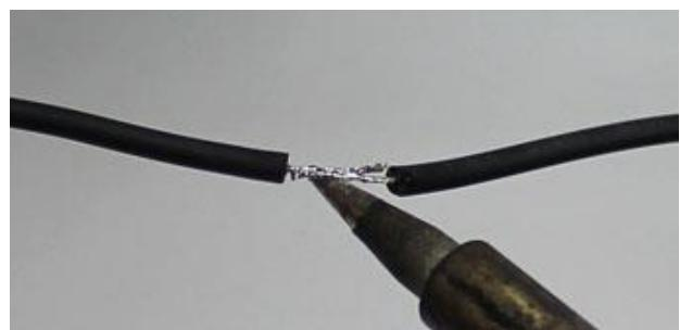
5. Remove the soldering iron and wait a few seconds to let the soldered connection cool and harden. Use heat shrink to cover the connection.
