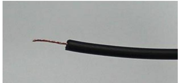
2. Make sure your soldering iron is fully heated and touch the tip to the end of one of the wires. Hold it on the wire for 3-4 seconds.
