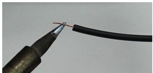
3. Keep the iron in place and touch the solder to the wire until it's fully coated. Repeat this process on the other wire.
