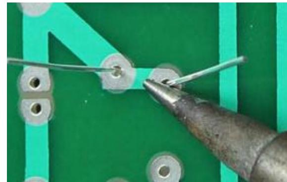
**Step 3: Apply Solder To Joint** – Continue holding the soldering iron on the copper pad and the lead and touch your solder to the joint. **IMPORTANT** – Don't touch the solder directly to the tip of the iron. You want the joint to be hot enough to melt the solder when it's touched. If the joint is too cold, it will form a bad connection.
