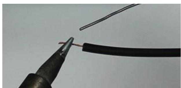
4. Hold the two tinned wires on top of each other and touch the soldering iron to both wires. This process should melt the solder and coat both wires evenly.
