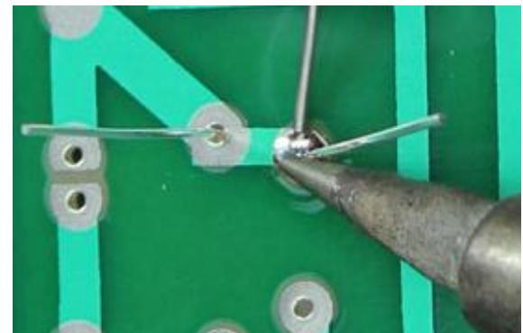
**Step 4: Snip The Leads** – Remove the soldering iron and let the solder cool down naturally. Don't blow on the solder as this will cause a bad joint. Once cool, you can snip the extra wire from leads.
